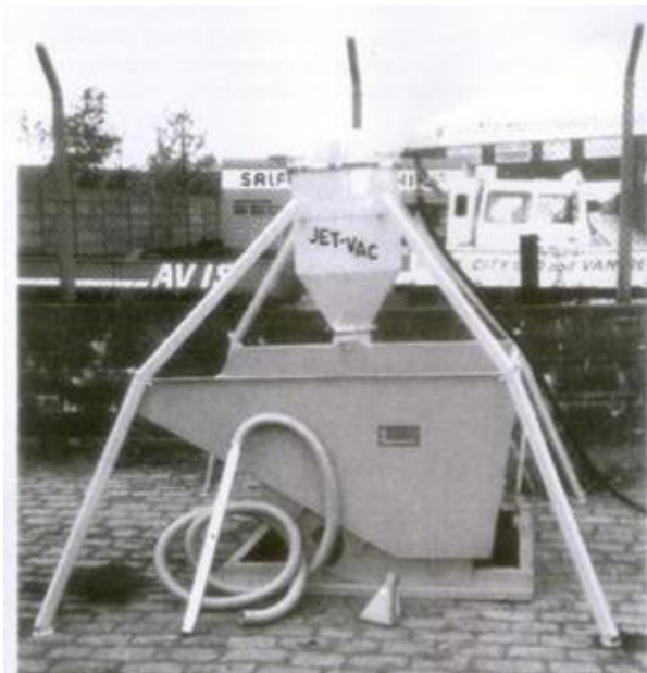
J.V.6 Lid Assembly unit with hopper & a clapper valve seated over a 2 cu. yd. skip with extension legs. Brackets can be manufactured to fit over any skip arrangement.
